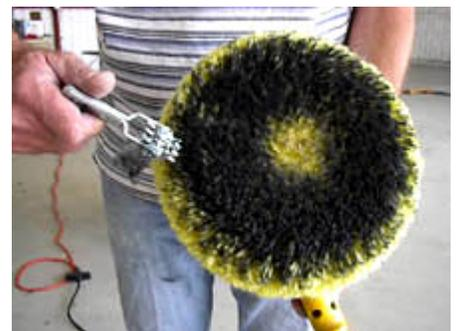
6. Add polish sparingly for subsequent passes. You will eventually develop a feel for when the pad is too dry. As a general rule, if you are seeing bright metal where the pad has been and are making very visible swirl marks, you are doing it right.
