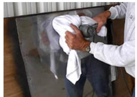
At this point take care to remove all residual polish from around rivet heads and seams. A solvent can be used but an old polishing technique of using cornstarch to remove residual polish is probably best. Read more about cleaning techniques at the end of the “Using the Cyclo Polisher” section.
