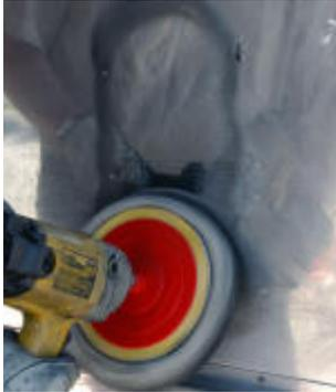
First Pass. Note the bright metal where the pad has been and that a line of polish has been deposited on either side of the pad.
