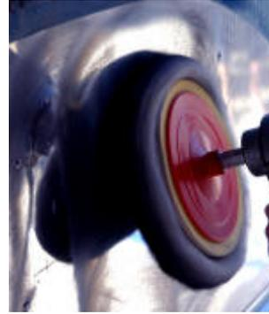
Start the second pass about 4" over from the first pass. Go down the line of polish that was deposited on the first pass. Make additional passes until you are working an area about 18" x 18".
