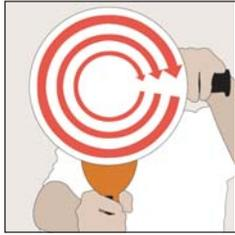
The outer rim of a single-spindle rotary polisher moves at a higher speed than the center. If a rotary polisher is held in one spot just a split-second too long, heat quickly builds up and causes burn marks. Smaller surface areas, such as curves and edges, are extremely vulnerable to this type of damaging heat. Rotary polishers are also known to bounce or skid across the work surface and to leave swirl marks.
